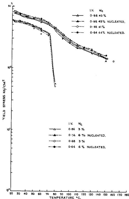
Figure 3 Variation of yield stress with temperature; effect of talc.
