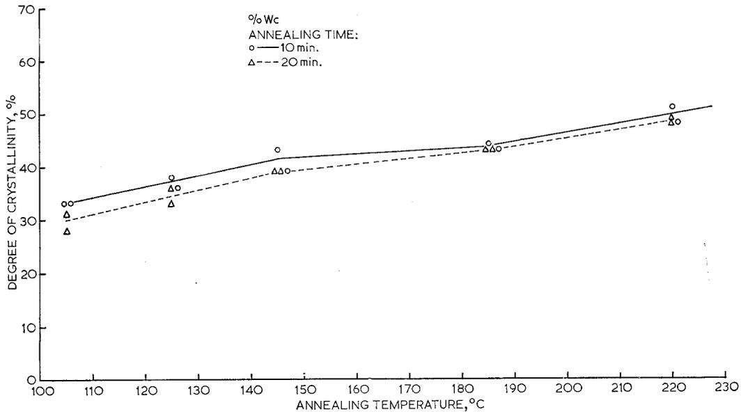
Figure 1 Variation of crystallinity with annealing temperature.
