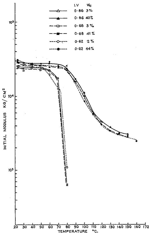
Figure 4 Variation of initial modulus with temperature; effect of crystallinity.
