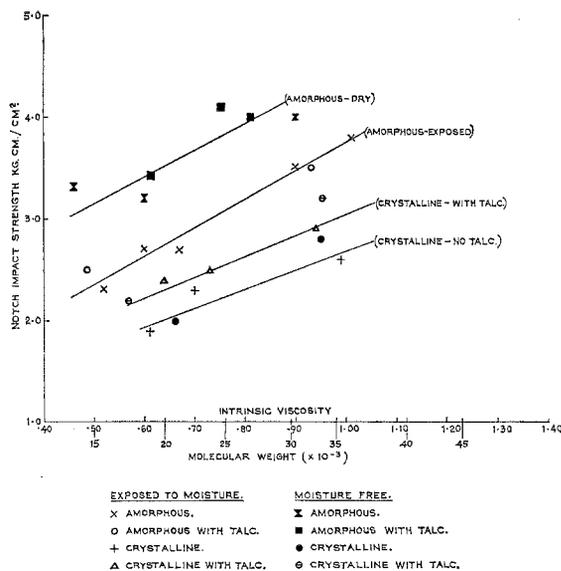
Figure 7 Variation of impact strength with crystallinity and intrinsic viscosity.
