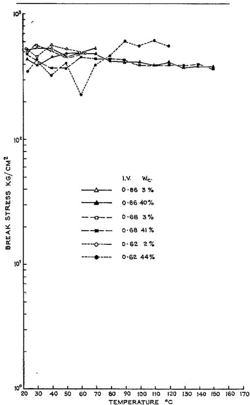
Figure 6 Variation of breaking stress with temperature.
