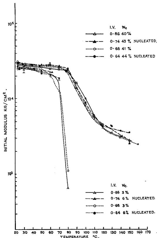
Figure 5 Variation of initial modulus with temperature; effect of talc.
