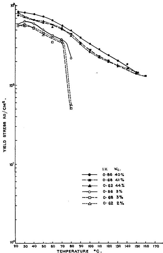
Figure 2 Variation of yield stress with temperature; effect of crystallinity.
